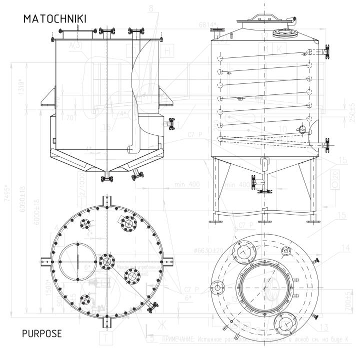
The matochnik of the EPP brand (version with a jacket, a mixing device) and MTCHK (with a coil) are used at the enterprises of the alcohol, food, livestock industries and are an element of the yeast growth department and are intended for growing yeast
