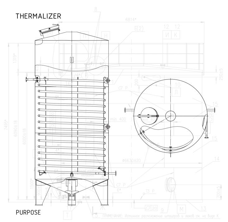
Tabi**Thermalizers** are part of the equipment for the production of dry fodder yeastumenobanue (Martin AX)
