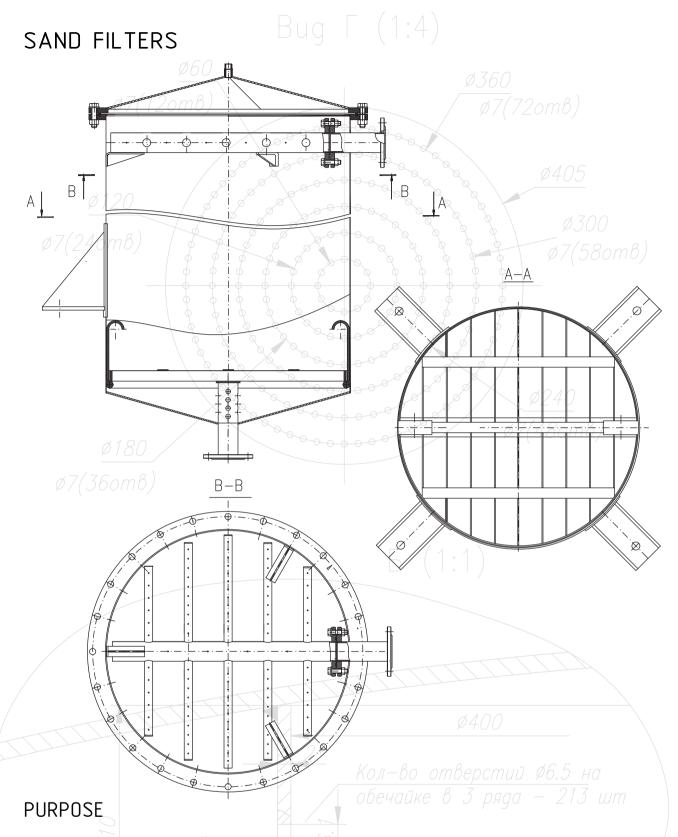
The equipment is intended for filtering water-alcohol and other solutions, cleaning the vapor-air mixture from inclusions after removing the juice vapors without condensation from the dryer into the aspiration system. Filters are used at the enterprises of the alcohol and wine-vodka industry and are installed in rooms that have category D in terms of explosion hazard.
