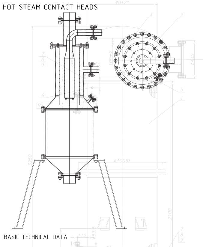
Equipment is a necessary element of the BRU rectification installation. Designed for steaming the mass, thermo-hydraulic processing of the batch.
