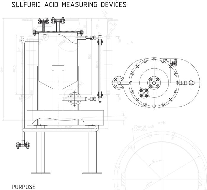
Sulfuric acid measuring tanks – technological tanks for storing production products, are a necessary element of the fermentation department of distilleries.
