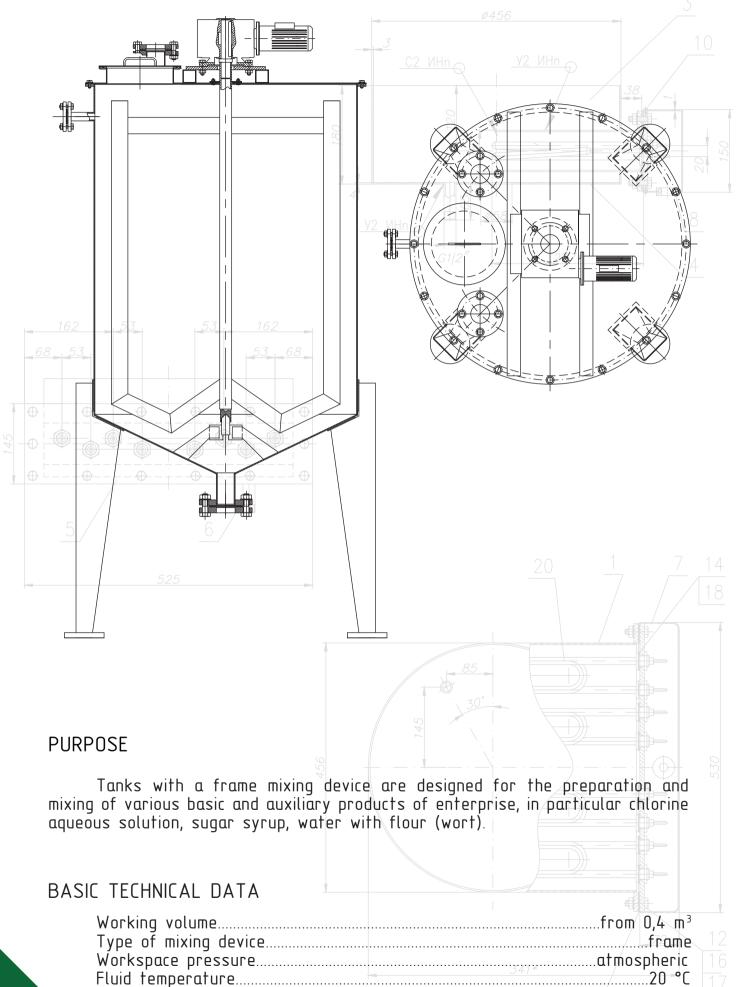
Material of construction......stainless or carbon steel
