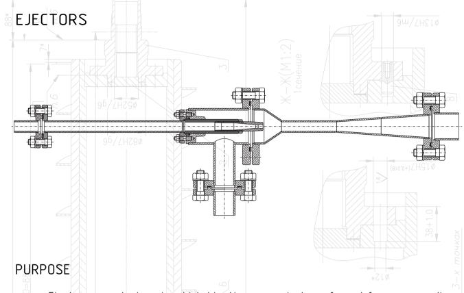
Ejectors are devices in which kinetic energy is transferred from one medium moving at a higher speed to another.
