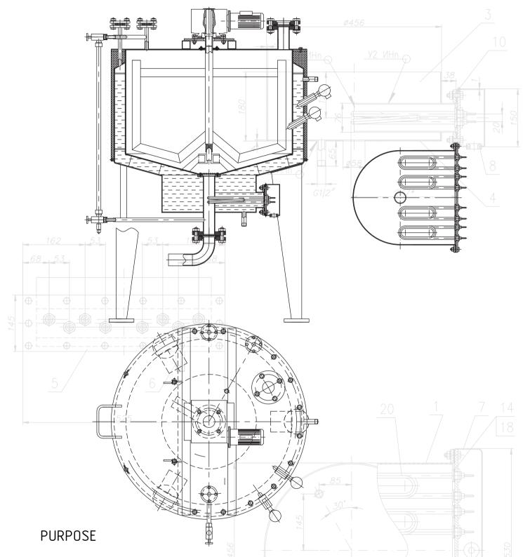
Tanks of this type are designed for the preparation of syrup in a hot way. As a mixing device, both paddle, frame and paddle mixers are used
