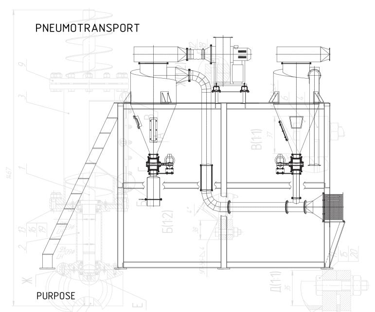
Pneumatic conveying units are a set of devices that facilitate the movement of bulk materials (dust, powder, granular, crushed, etc.) using compressed air or discharged gas. With granules of transported material up to 10 mm, pneumatic transport is preferable in almost all cases to other transport systems.
