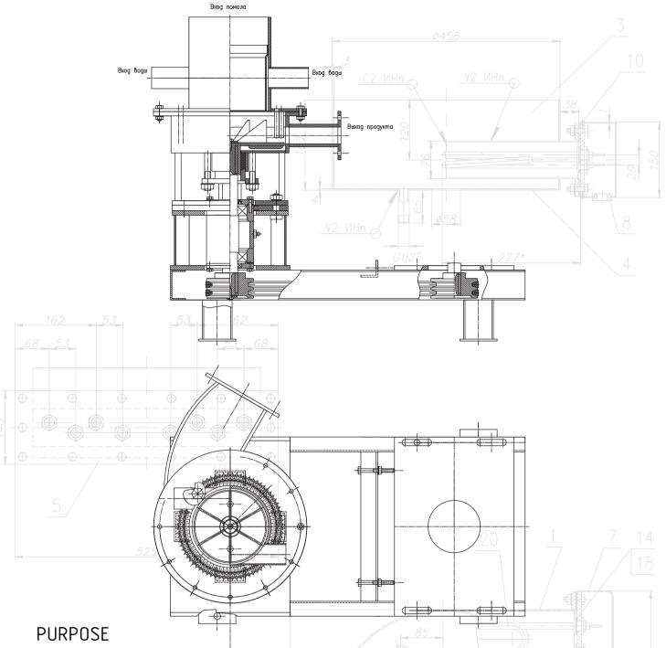
The mixing equipment is designed to mix the grinding product with a liquid, to prepare wort with a solids content of up to 22%, in particular for preliminary mixing of crushed grain with water.
