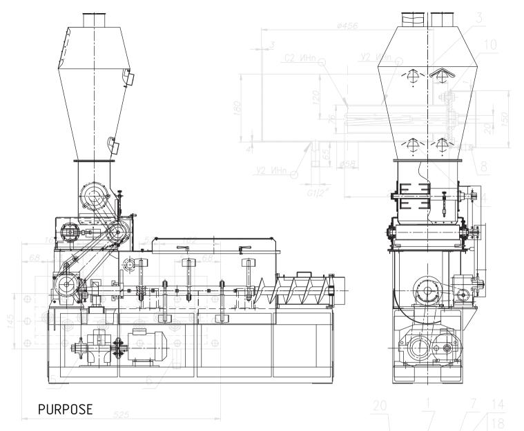
Continuous dough mixing plants with a one- or two-component receiving hopper have a stationary cylindrical horizontal kneading tank and a kneading shaft located in it with a blade mixing device passing into the unloading auger.
