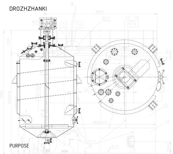
Drozhzhanki are designed for growing yeast and are a cylindrical apparatus with a conical lid and bottom, equipped with a paddle mixers
