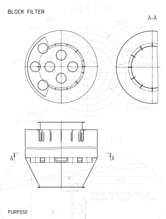
Block filters are designed to clean the vapor-air mixture from inclusions after the output of juice vapors without condensation from the dryer into the aspiration system.
