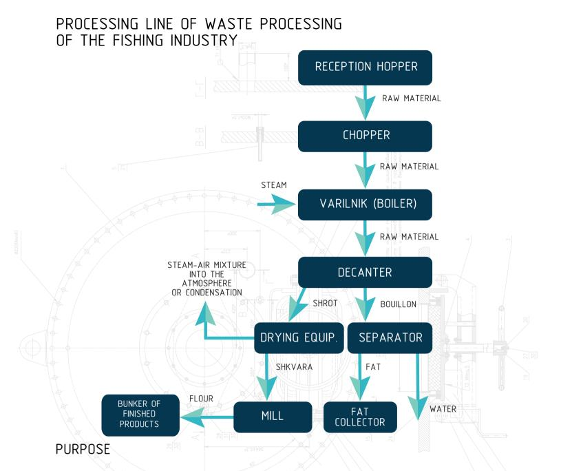
Technological lines for the high-temperature processing of waste from the fishing industry are intended for the production of compound feed (fish meal) and technical fat.
