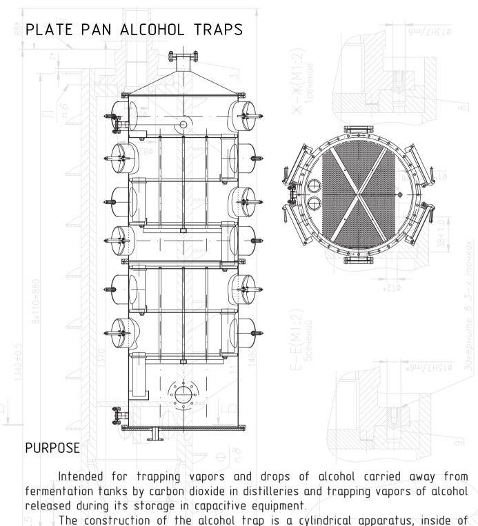
which six sieve plates are placed at equal distances.
