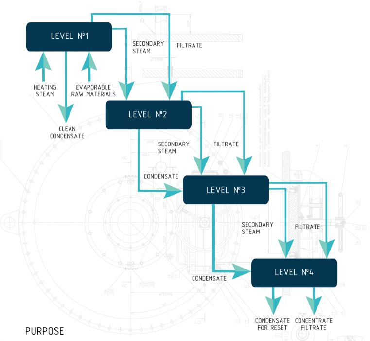
It is intended for evaporation and drying of raw materials in the agricultural, fish processing, meat processing, alcohol industries: obtaining juice, wine concentrates, adhesive broth concentrate, tomato paste production, evaporation of alcohol stillage filtrates (vacuum-evaporating multi-unit plants, bardo-dewatering plants).
