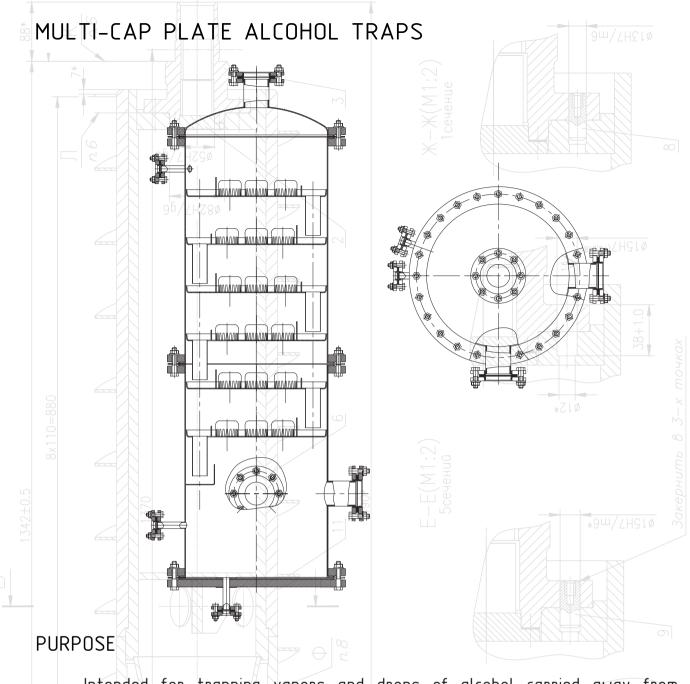
Intended for trapping vapors and drops of alcohol carried away from fermentation tanks by carbon dioxide in distilleries and trapping vapors of alcohol released during its storage in capacitive equipment.
