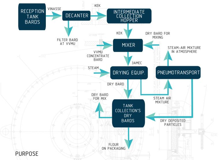
Drying lines for post-alcohol stillage are designed for the production of animal feed.
