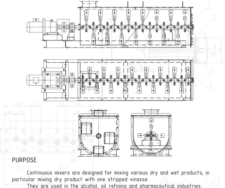
The mixer consists of a cylindrical body, a shaft with blades, inlet and outlet pipes and hinged covers. The mixer body is welded to the bed. The shaft is mounted in bearing, mounted in cups at the ends of the housing. On the shaft are blades with different angles of rotation relative to the plane perpendicular to the axis of the shaft. The shaft is driven by an electric motor through a belt drive.
