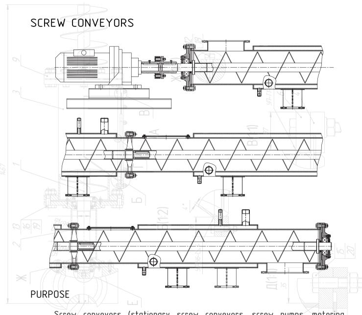
Screw conveyors (stationary screw conveyors, screw pumps, metering augers) are designed for transportation in horizontal and inclined (at an angle of up to 40°) positions, at temperatures up to 80°C dusty, powdery, small-sized (piece size up to 20 mm), non-abrasive and abrasive bulk cargo.
